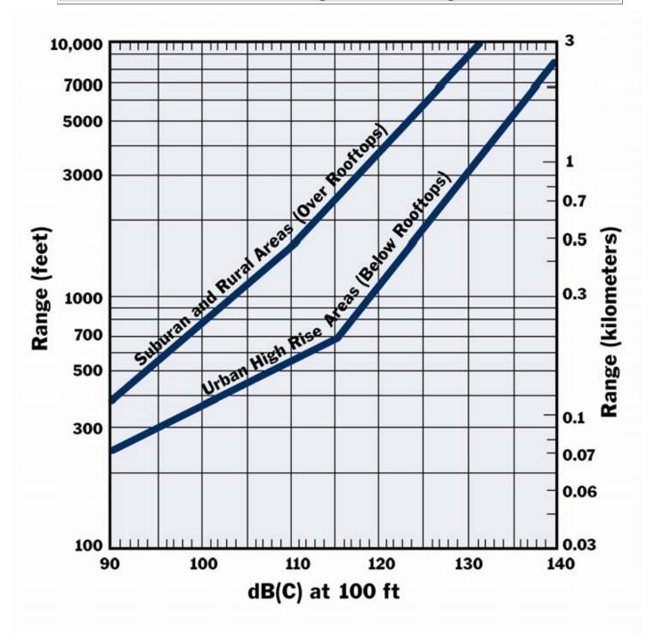
Figure F-1: Rated Output of Warning Device in dB at 100 feet
